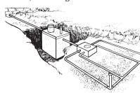
**Cesspool:** a buried chamber such as a metal tank, perforated concrete vault, or covered excavation that receives wastewater or sanitary sewage to be collected or discharged to the surrounding soil.
